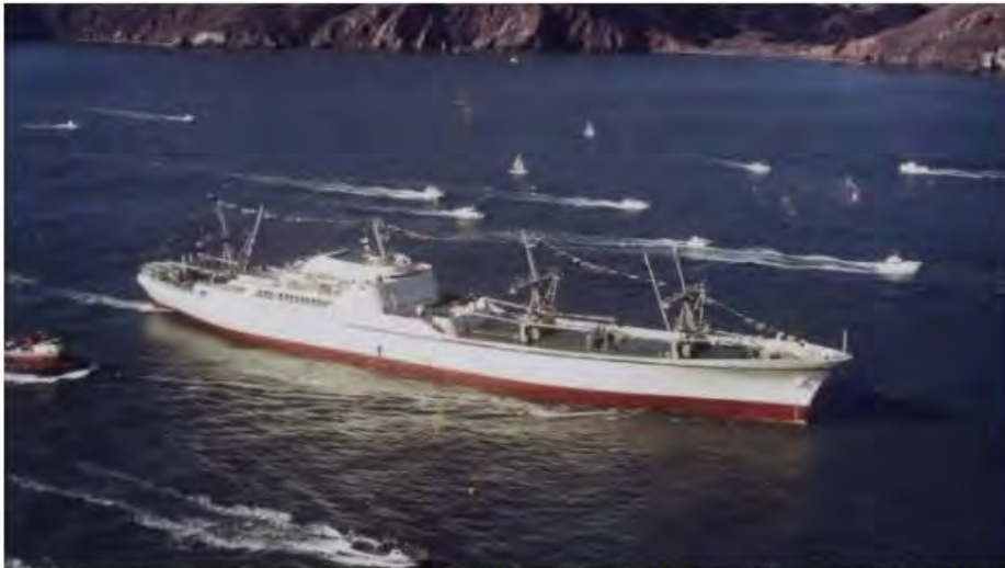
NS Savannah operated in the 1960s as the US's first demonstration of nuclear power on a merchant ship (Nuclear Regulatory Commission photo)
